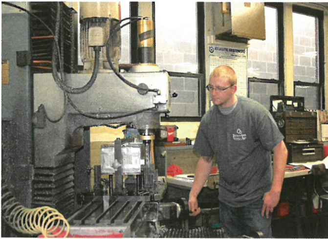
Manual milling with Proto-Trak controller is possible since all machine operators are trained machinists.
