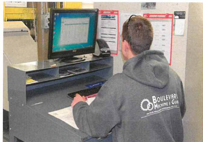
A machine operator scanning a traveler into the Job Boss program. Boulevard can live track every job in the shop giving them up-to-date progress through each work center.
