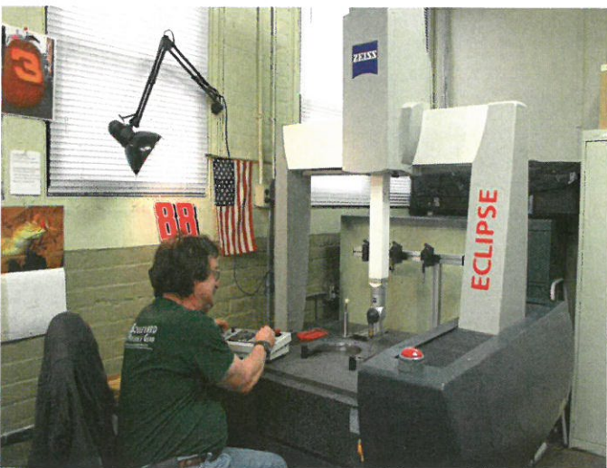
This Eclipse CMM unit is just one of a couple quality control ways of insuring every part that leaves Boulevard is 100% in tolerance. Look at the complicated part that they checked with this machine!
